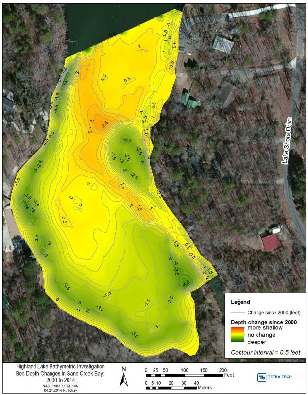
Figure 7. Changes in depth between 2000 and 2014, Sand Creek Bay.
