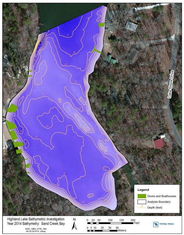
Figure 4. Sand Creek Bay bathymetry surveyed in March 2014.
