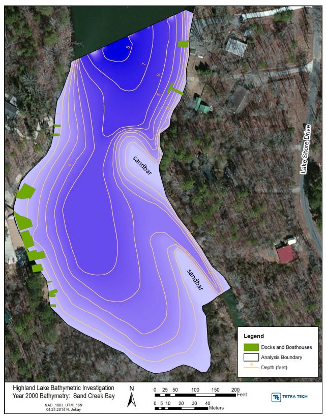
Figure 3. Sand Creek Bay bathymetry surveyed in 2000 before dredging.
