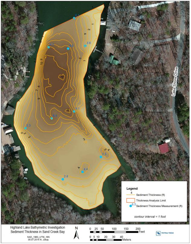
Figure 9. Sediment thickness in Sand Creek Bay.
