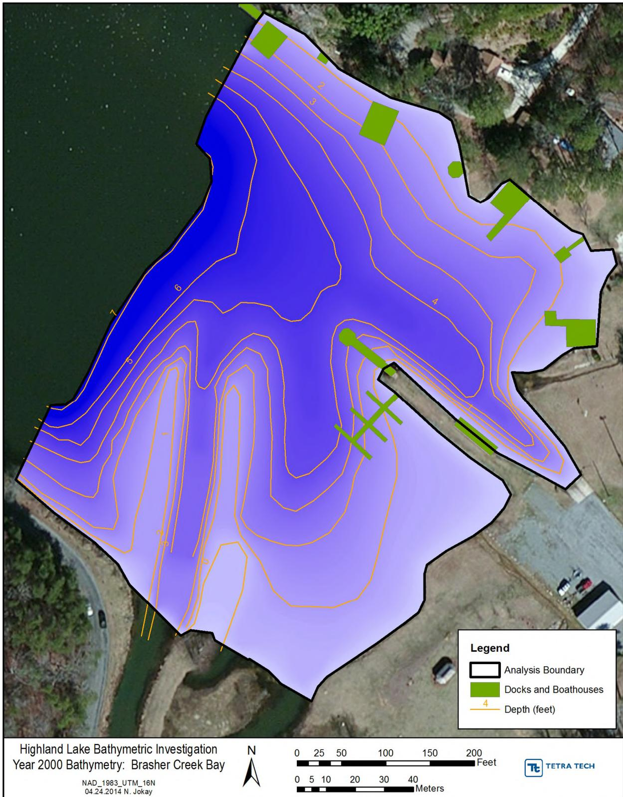
Figure 1. Brasher Creek Bay bathymetry surveyed in 2000 before dredging.
