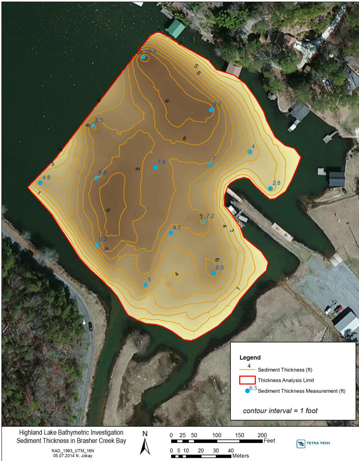
Figure 8. Sediment thickness in Brasher Creek Bay.
